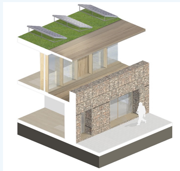
Figure 3.8 Axonometric of the gateway building facade
